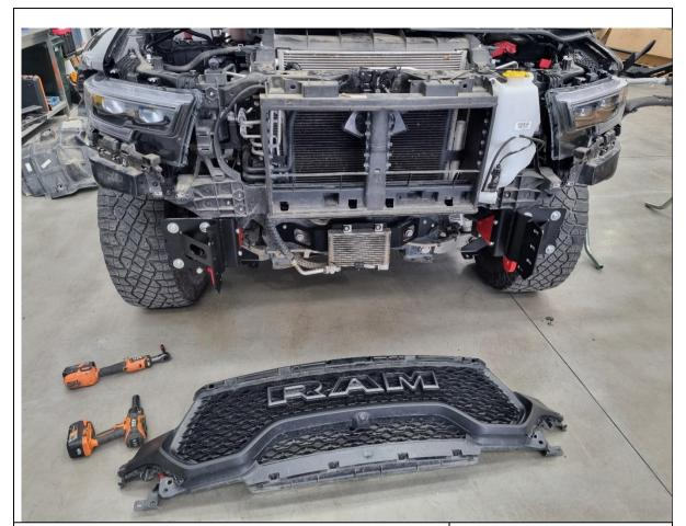
18. Lift upwards and outwards to remove the grille.
