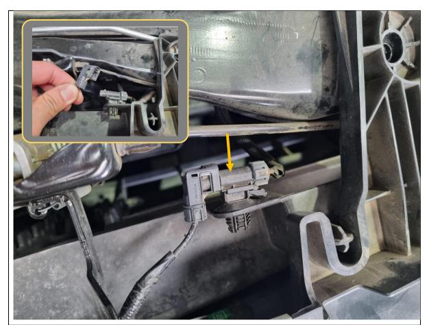
17. Locate the camera plug on top of the grille, below where the radiator cover was. Press down on the connector tab and disconnect the camera harness.
