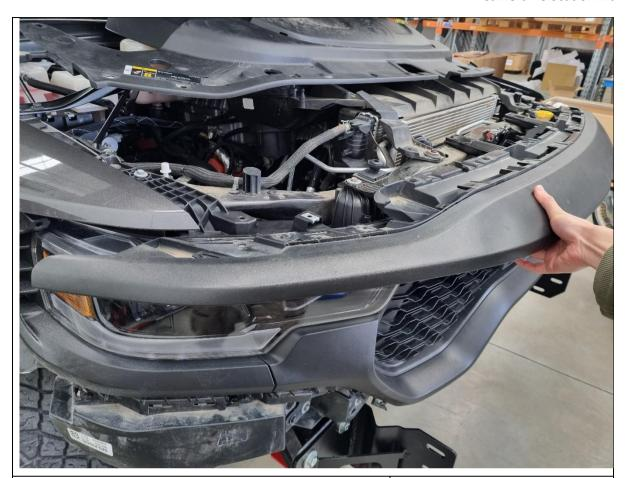
6. Once all clips and bolts are removed, pull outwards to remove the grille top trim and set aside for refitment.
