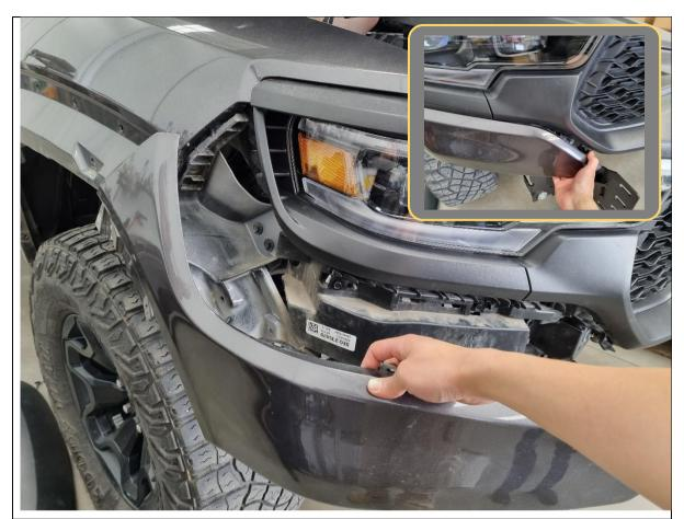
12. Remove the plastic trim under each headlight. Start at the base of the grille and pull the trim outwards to release the clips.
